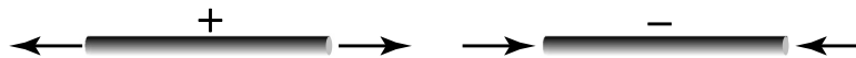
Fig. 23. This is the convention used in the books on strength of materials.
